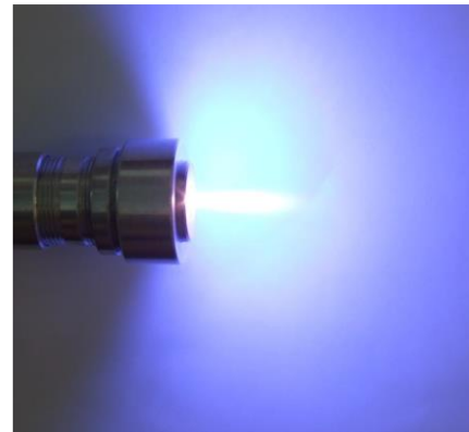
800W plasma Jet for air cleaning, activation and more
