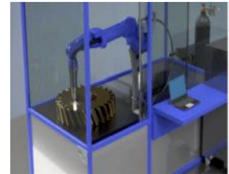
500W Plasma jet driven for 3-D printing
