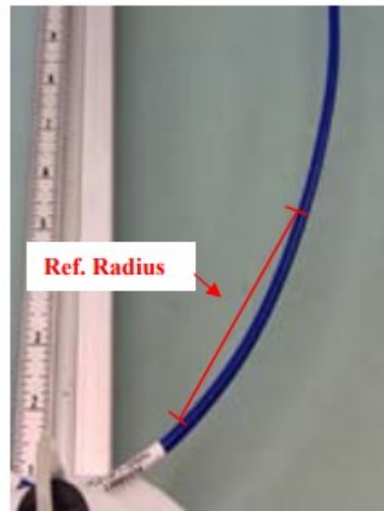
Figure 2: 3ft. Flexible Test Cable attached to the Cable Flexure Test Fixture at its reference start position
