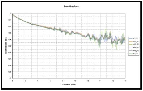
Fig. 8 Insertion Loss DUT 02
