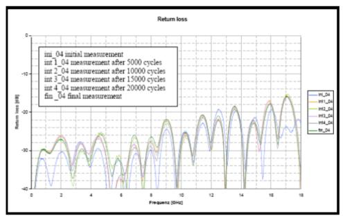
Fig. 11 Return Loss DUT 04
