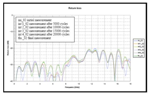
Fig. 7 Return Loss DUT 02
