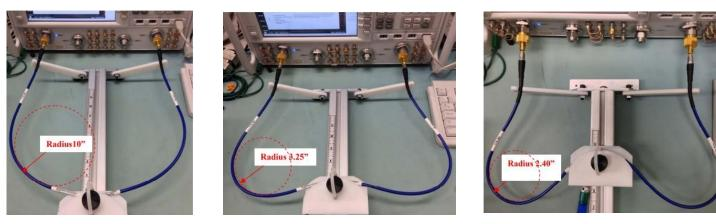
Figure 1: "Cross Bow" apparatus for measuring cable performance versus bend at 10", 3.25", and 2.4" bend radii.
