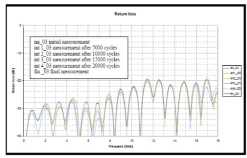
Fig. 9 Return Loss DUT 03
