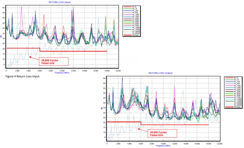
Figure 5 Return Loss-Output
