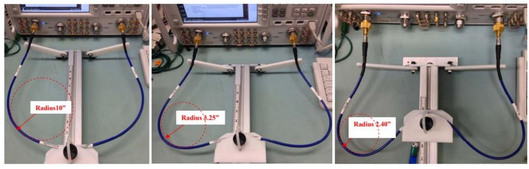
Figure 3: 3ft. Flexible Test Cable with a bend radius of 10"
