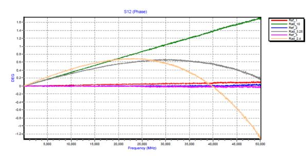
Figure 2: T50-3FT-KMKM+ using the "cross-bow" two port method, exhibiting a parabolic relationship between phase change and flexure.
