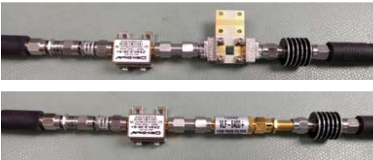
Figure 15: (top) A reflectionless filter and doubler pair. (bottom) A reflective filter and doubler pair.
