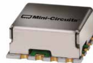
Figure 5: Model ROS-4608CH-2+ is a surface-mount VCO with fixed-frequency output at 4608 MHz with typical tuning sensitivity of 6 MHz/V for a control voltage range of 0.9 to 4.35V
