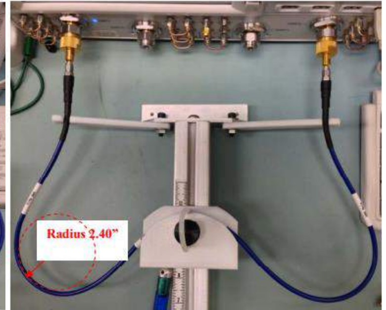
Figure 5: 3ft. Flexible Test Cable with a bend radius of 2.40"
