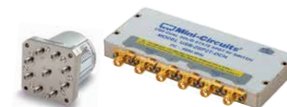
Figure 1: SP8T electromechanical switch, MSP8T-12D+ (left), and dual SPDT solid state switch, USB-2SP2T-DCH (right). No single switch design meets all test needs. Tradeoffs are often required on performance, speed, and number of switching cycles
